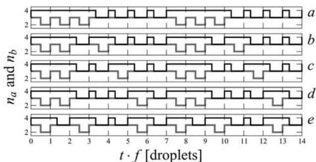
**Fig. 5** Number of droplets in the right channel ( $n_a$ , values between 2 and 3) and left channel ( $n_b$ , between 3 and 4) as a function of time. The loop has arms of length 2 mm (left channel) and 2.1 mm (right channel) and the droplet equivalent length is 0.2 mm, the parameters correspond to the point ( $f = 250$  Hz,  $L_a = 2.1$  mm) in Fig. 4. Shown are all five patterns available for this point of parameter space: RRRLLLL (a), RRLRLLL (b), RRLRLRL (c), RRLRLRL (d), RLRLRLL (e).
